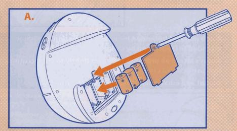
Use a Phillips/cross head screwdriver (not included) to loosen screw in battery compartment door. Insert 3 x 1.5V C or LR14 size batteries. Alkaline batteries required. Replace door and tighten screw.
