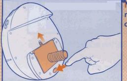
**NOTE** Push button and slide crib mount panel to access battery compartment.
